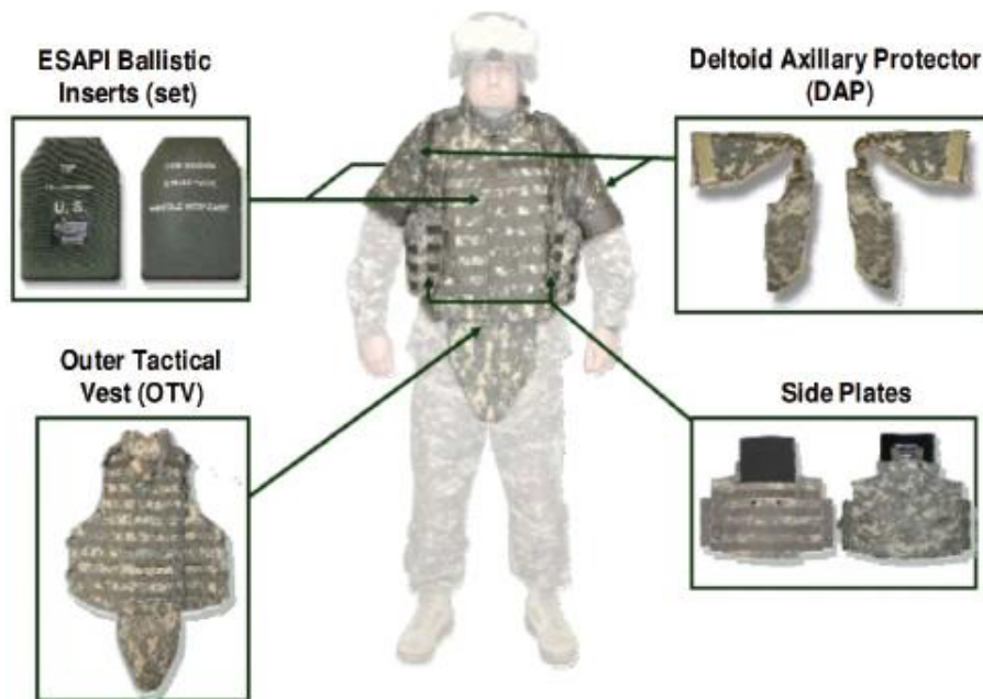
FIGURE 2-5 Interceptor body armor. Shown are the various components that make up the Interceptor body armor system (see DoD Inspector General’s Report No. D-2009-047, January 29, 2009). The outer tactical vest, the deltoid axillary protectors, and the carrier for the ESAPI inserts (not shown) are made of Cordura, Kevlar, and/or Twaron fabric. The ESAPI ballistic inserts are composite ceramic plates
