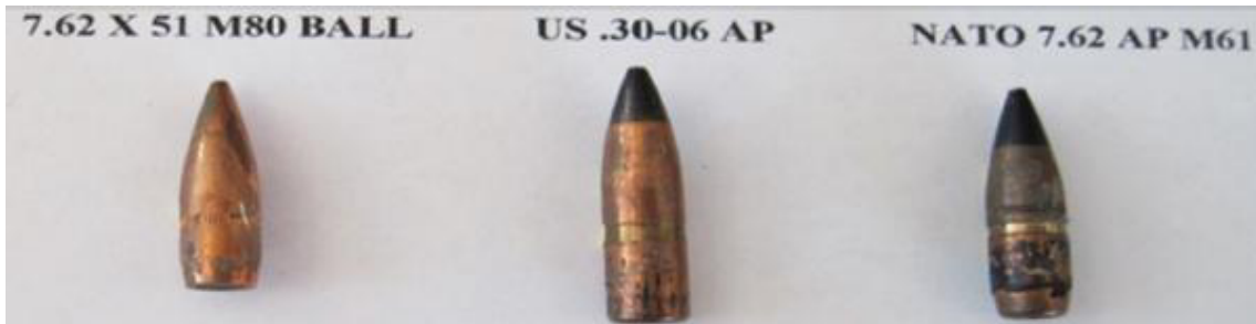
FIGURE 2-3 Examples of 7.62 mm (.30 cal) small arms projectiles. SOURCE: Courtesy of Robert Skaggs.
