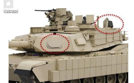
The system employs actively scanned radar to provide continuous 360-degree protection of the vehicle. Radar is considerably superior to other sensors as a primary threat detector due to its greater effectiveness in adverse combat conditions like smoke, sand, dust, mud, glare and battlefield explosions. U.S. Army requirements demand that an APS must be capable of protecting vehicles under all conditions.
