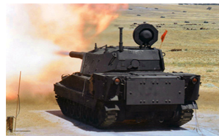
The FMC Close Combat Vehicle-Light ultimately won the AGS contest. Here a pre-production XM8 fires its 105 mm main gun.
