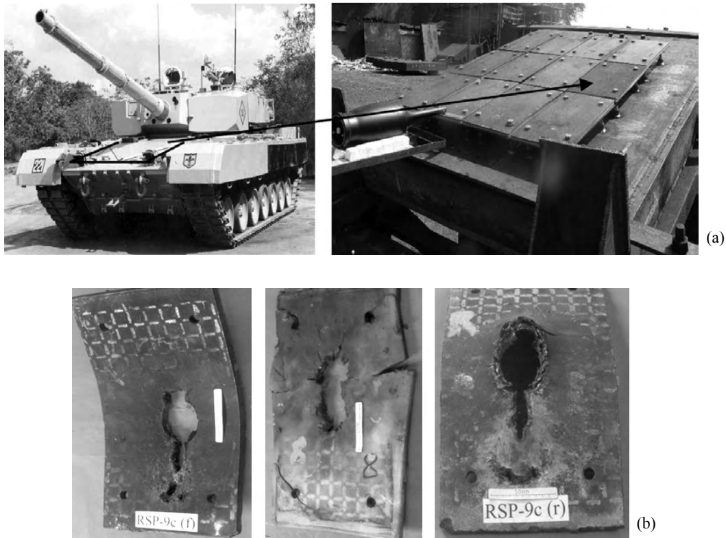
Figure 7. Ballistic evaluation of dynamic passive armour against HEAT missile: (a) test set-up, and (b) damage of the cassette material.
