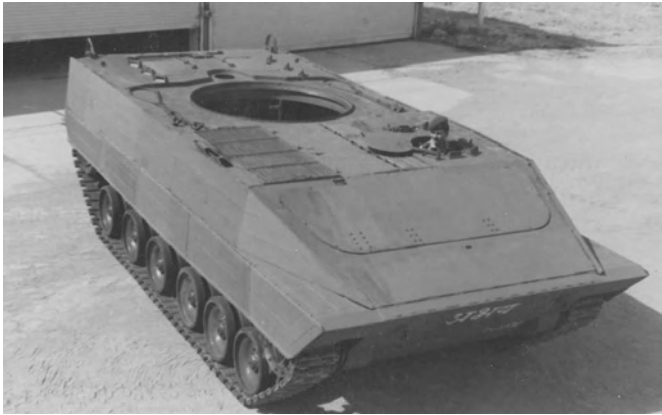
Figure 4. Experimental infantry combat vehicle with appliqué VHS armour visible on the glacis.
