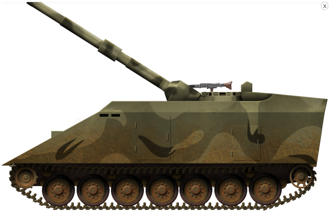
Illustration of the FCM New Start Howitzer Improvement Program, showing the forward placed driver compartment connected to the rear fixed superstructure. Illustration by Yuvnashva Sharma, funded by our Patreon campaign.
