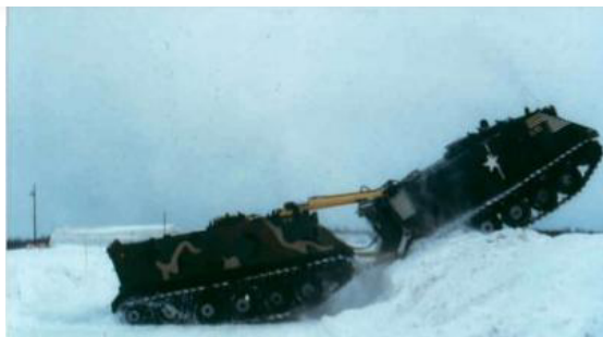
M113 CCRV project during snow trials. The vehicle could be controlled from either front or rear vehicle. Source: TACOM/TARDEC
