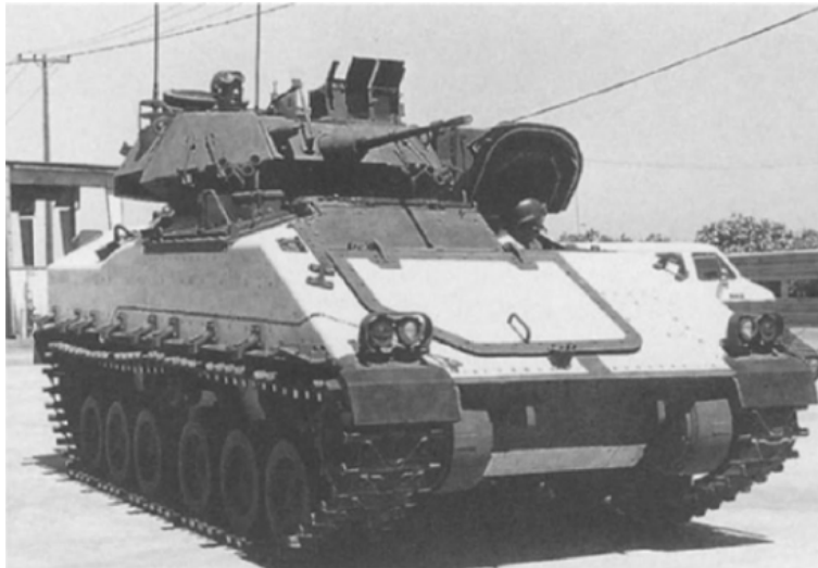
Composite-hulled M2 Bradley Infantry Fighting Vehicle with non-composite turret. Source: Pilato and Michno
