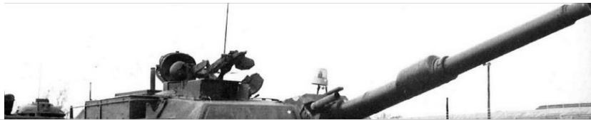
One of the 14 M1E1s as fitted with the XM256 120 mm smoothbore gun and other improvements, including substantial slabs of steel welded to the hull and turret front to mock up the weight of a new armor package. Source: Mesko
