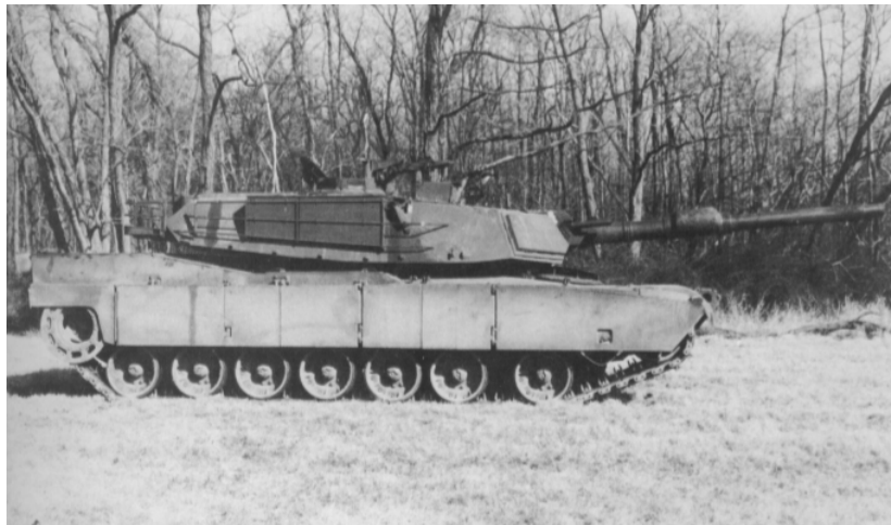
M1E1 first pilot model built in March 1981. Note the wide ring fitted around the rear sprocket in an effort to prevent it from throwing tracks. Source: Hunnicutt
