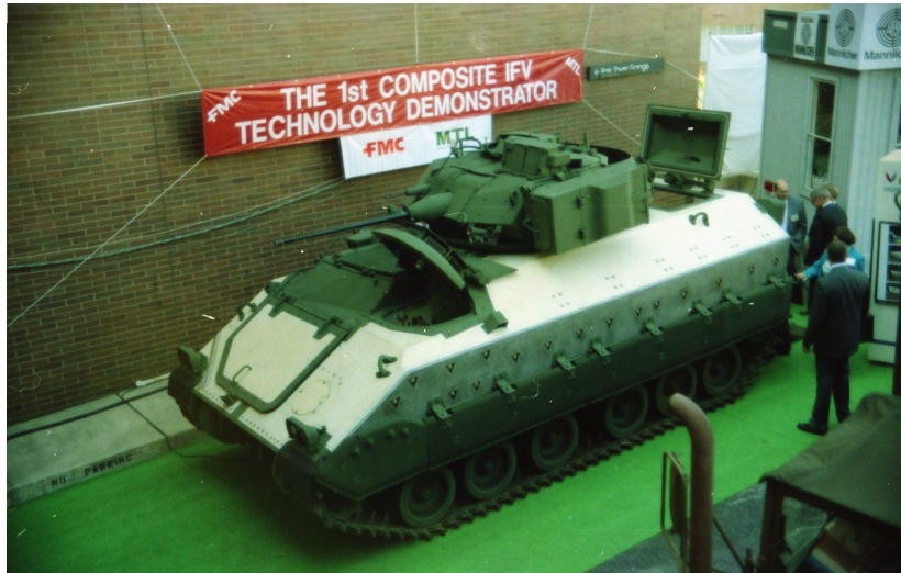
Unveiling and examination of the composite hulled Bradley at AUSA. Source: Richard Eshleman'
