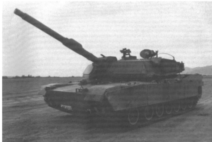
One of the 14 M1E1s as fitted with the XM256 120 mm smoothbore gun and other improvements, including substantial slabs of steel welded to the hull and turret front to mock up the weight of a new armor package. Source: Mesko
