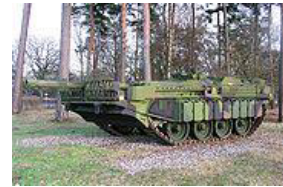
Swedish Stridsvagn 103 was designed to nearly disappear in a hull-down position.
