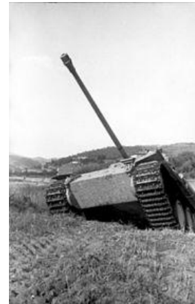
A tank's exposed belly armour is vulnerable to even modest antitank weapons. This is a Panther tank, cresting a hill.
