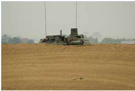
Leclerc tank in a hull-down position. Note the observation periscope which would allow the commander to observe in turret-down position.
