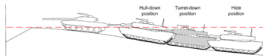
An M1 Abrams tank in hull-down, turret-down, and hidden positions behind a crest of ground. Shown to the left is the more exposed hull-down position a T-72 must adopt because of its main gun's limited range of depression (five degrees vs. the M1's ten degrees).
