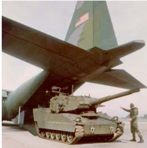
Loading the M-8 Ridgeway Armored Gun System for air transport.
