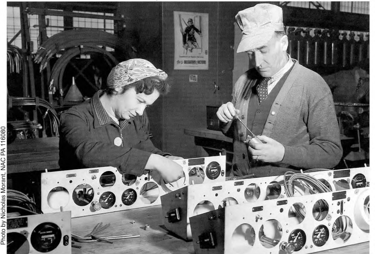
Male and female workers assemble instrument panels for Ram tanks at the Montreal Locomotive Works Plant, 1942.
