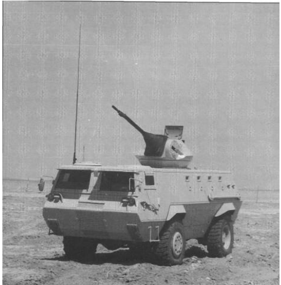
One of the many variants of the Fahd APC, seen here armed with a 20 mm cannon turret
