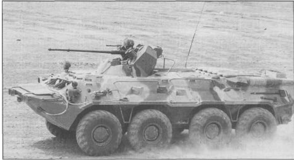
The external 30 mm cannon marks this BTR-80 model as the BTR-80A.
