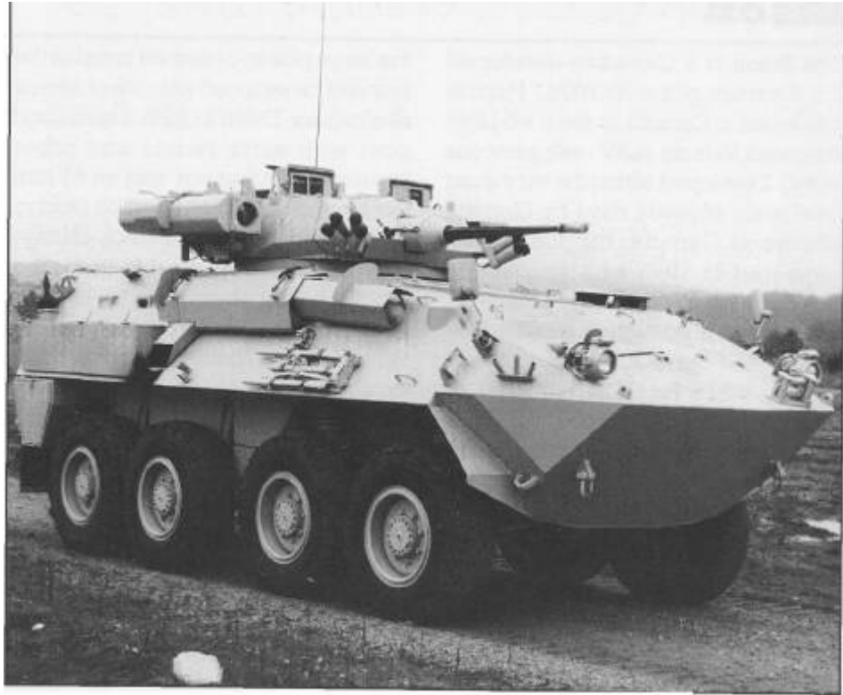
The LAV-25IFV, base model of the Light Armoured Vehicle (LAV) family.
