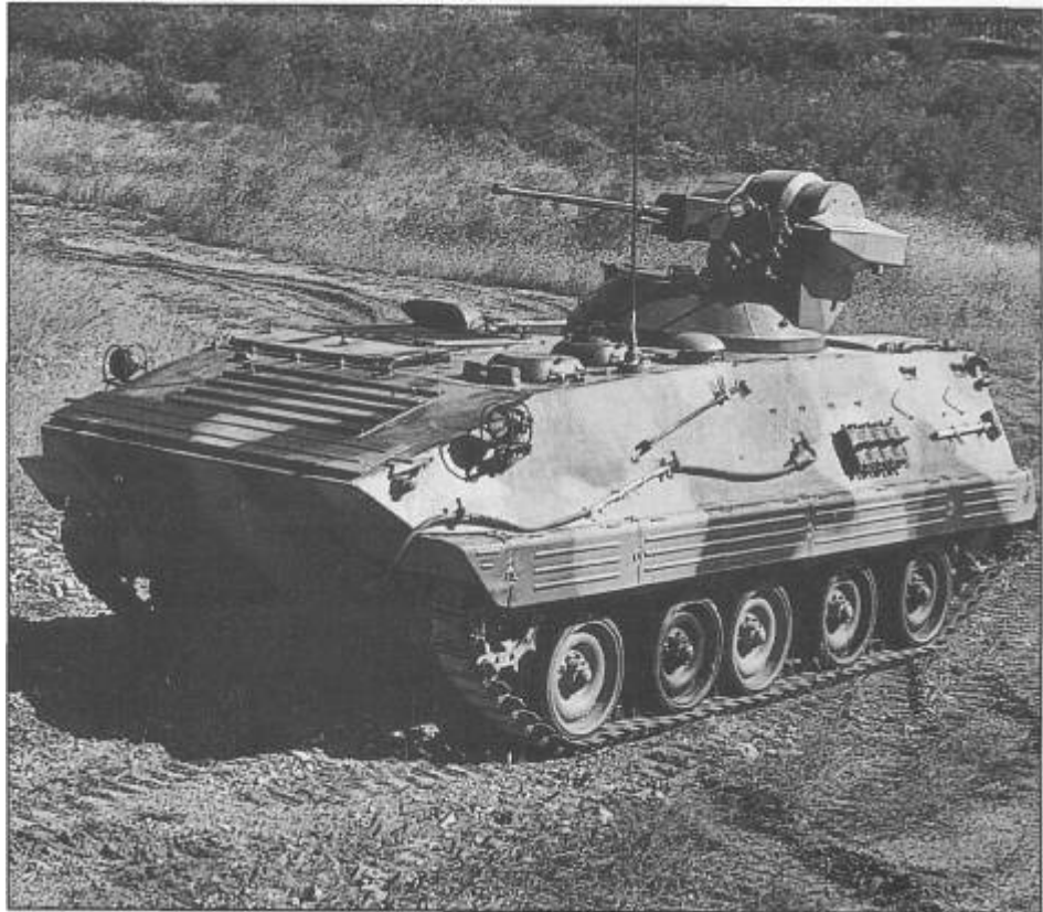
The external 25 mm cannon marks this IFV as the YW 307, the IFV model of the Type YW 534 family.
