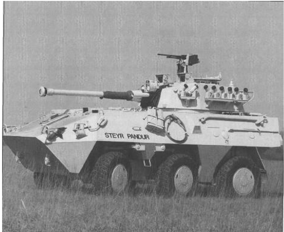
The Steyr Pandur configured as a reconnaissance vehicle armed with a 90 mm gun.
