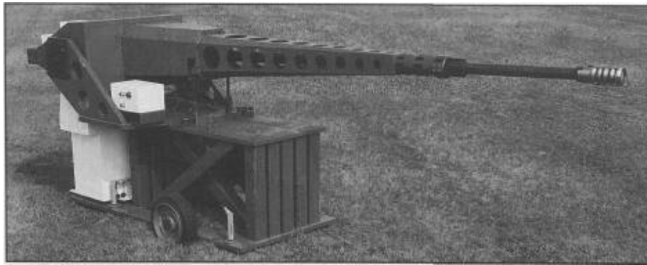
Below: A glance into the future, the proposed French - British 45 mm gun designed to fire CTA ammunition and destined for the next generation of IFVs.
