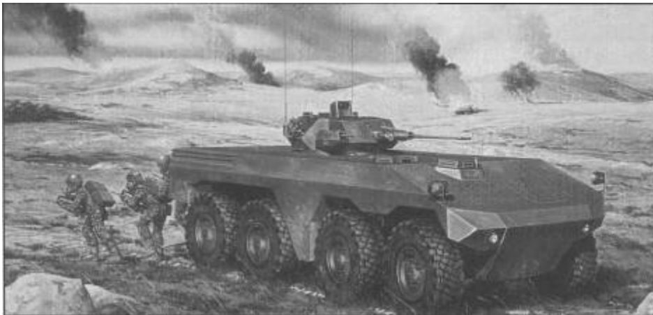
Above: A vision of the future - troops leaving a future French 8x8 IFV design armed with a 30 mm cannon.
