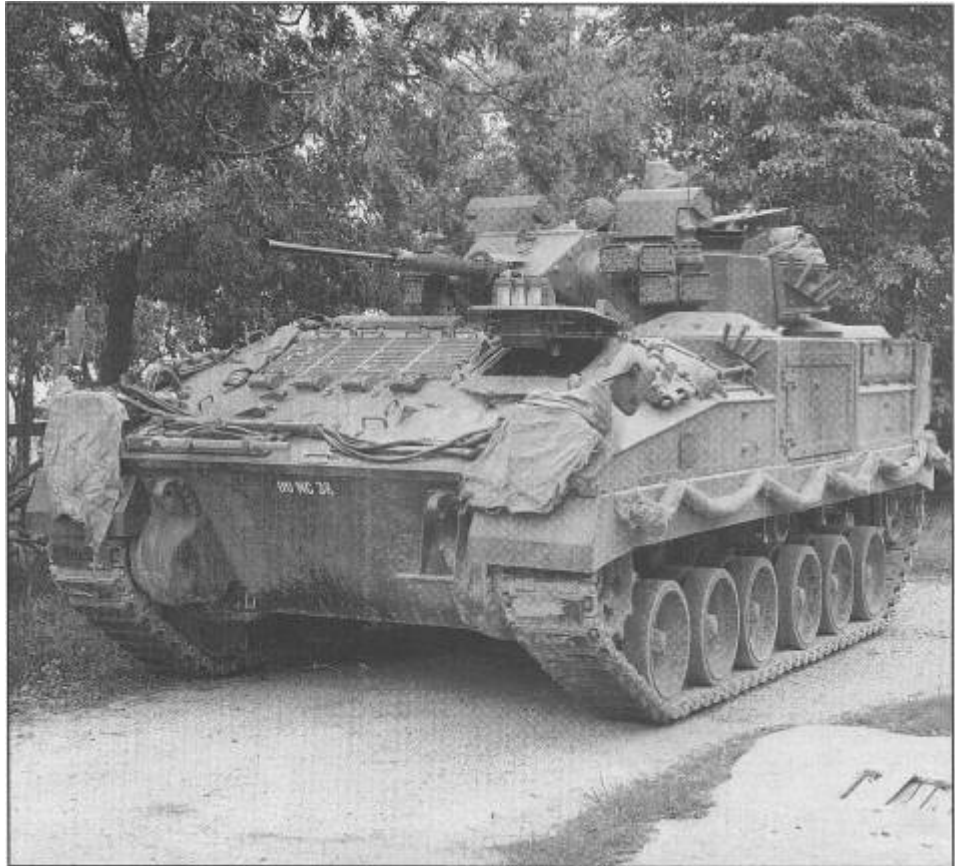
A Warrior IFV lacking the 'full combat' additional side armour as used in The Gulf.
