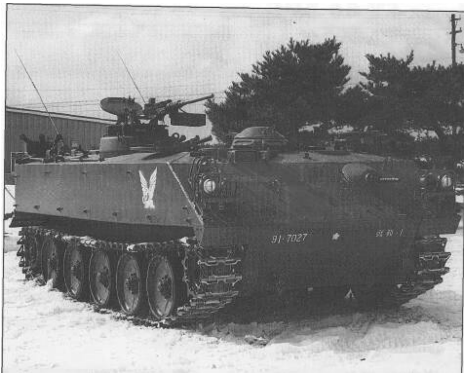
The Japanese Type 73APC-note the hull NIC,
