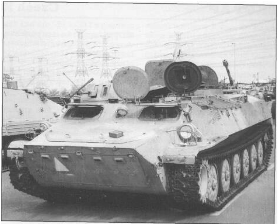
A captured Iraqi Army MT-LBAPC, a versatile and much-used general purpose carrier.
