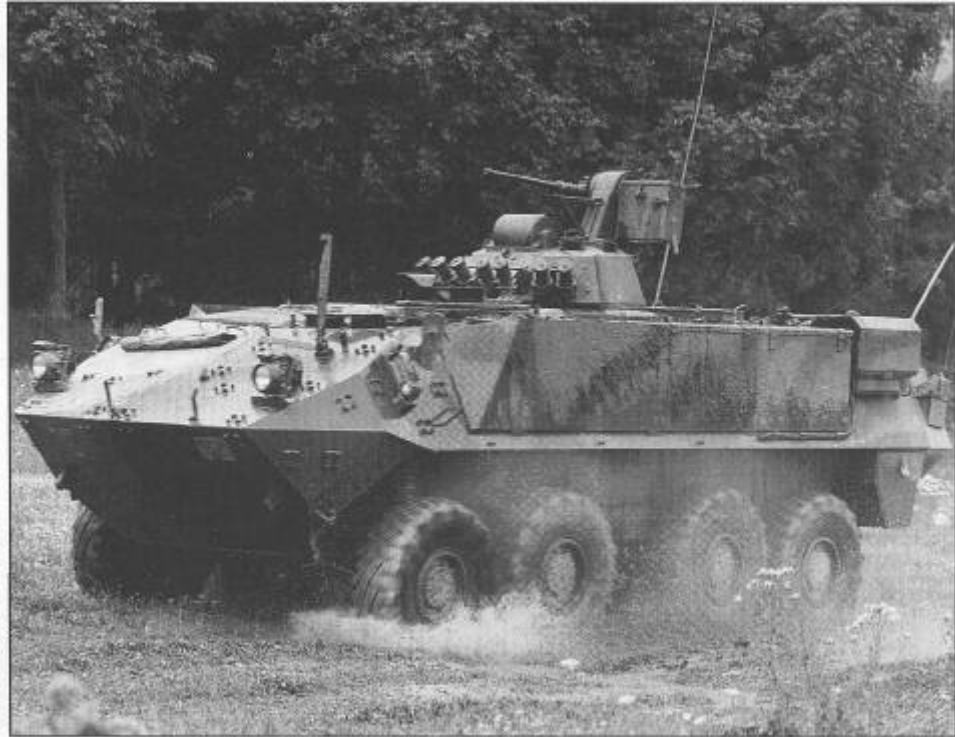
An 8 x 8 model of the Piranha APC armed with an externally mounted 12.7 mm MG.
