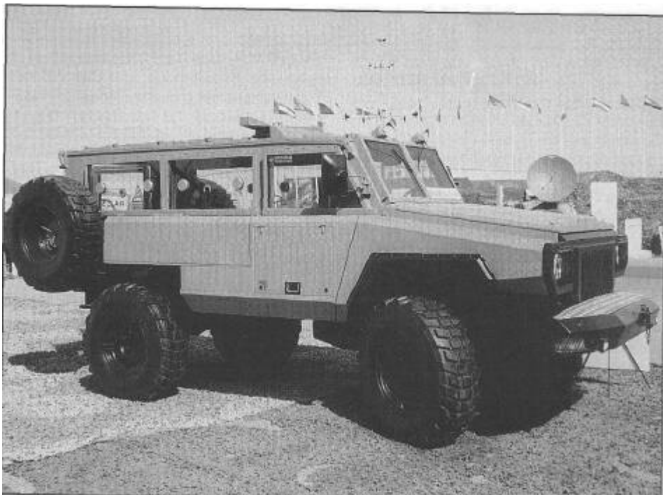
The mine-protected Mamba 4x4 APC, shown here unarmed.
