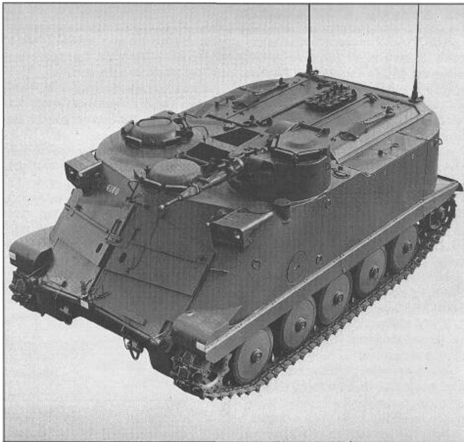
The Swedish Pbv302 APC, one of the first APCs to be armed with a 20mm cannon as standard.
