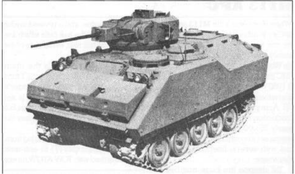
The FMC Armoured Infantry Fighting Vehicle (AIFV), produced in several forms in various countries.
