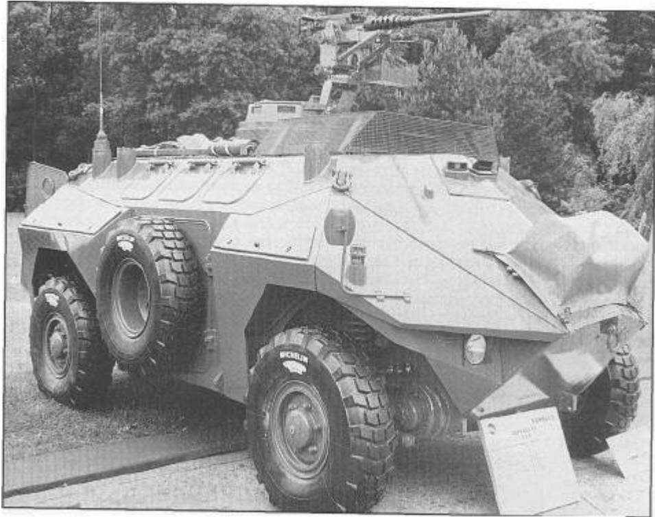
The Panhard Buffalo APC, showing its resemblance to the Panhard M3 from which it was developed.
