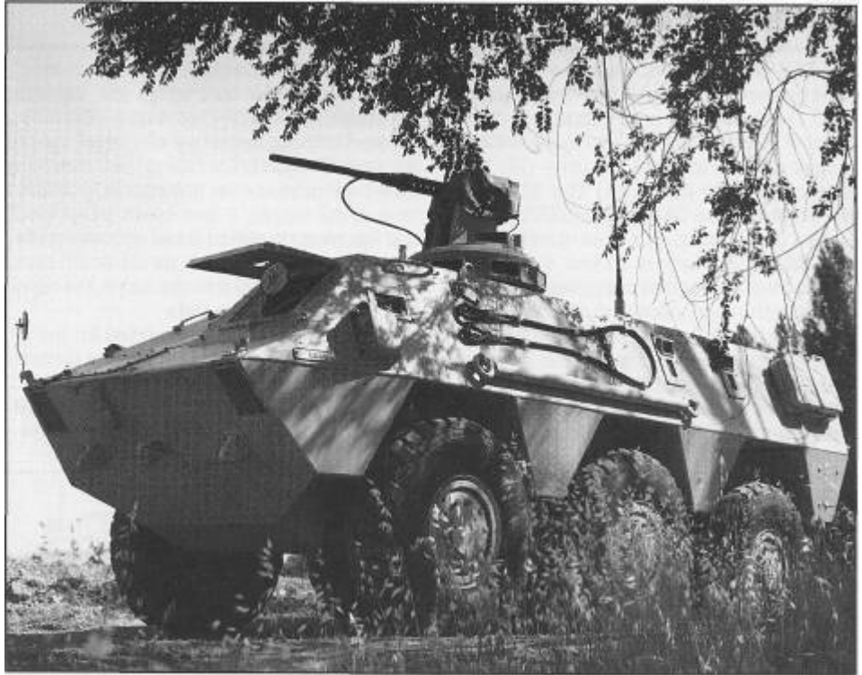
Spain's BMR-600 wheeled IFV seen here armed with an externally-mounted 12.7mm MG.
