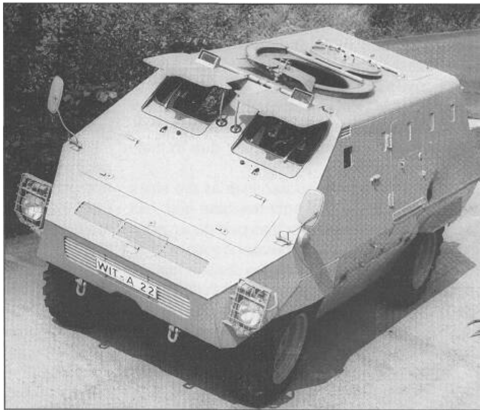
The UR-416 wheeled APC, basically a Unimog truck chassis with an armoured body.
