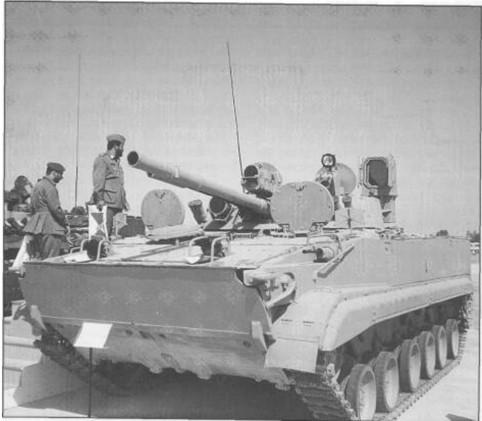
The bulk of the BMP-3 IFV can be appreciated in this view - note the hull-mounted MG.
