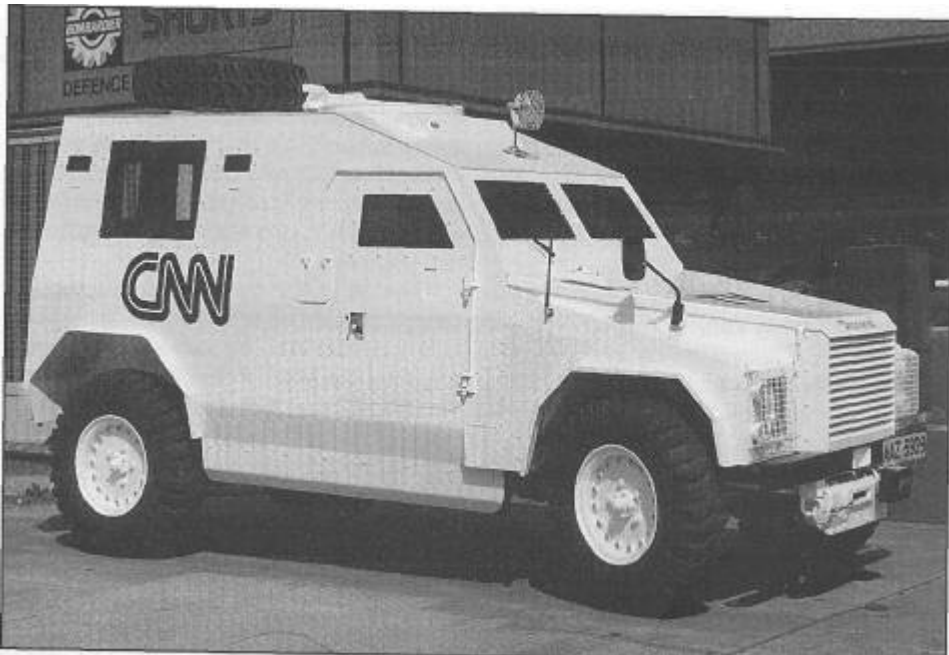
A Shorland wheeled APC in 'ciwie' guise as an armoured carrier for CNN television crews operating in Bosnia.
