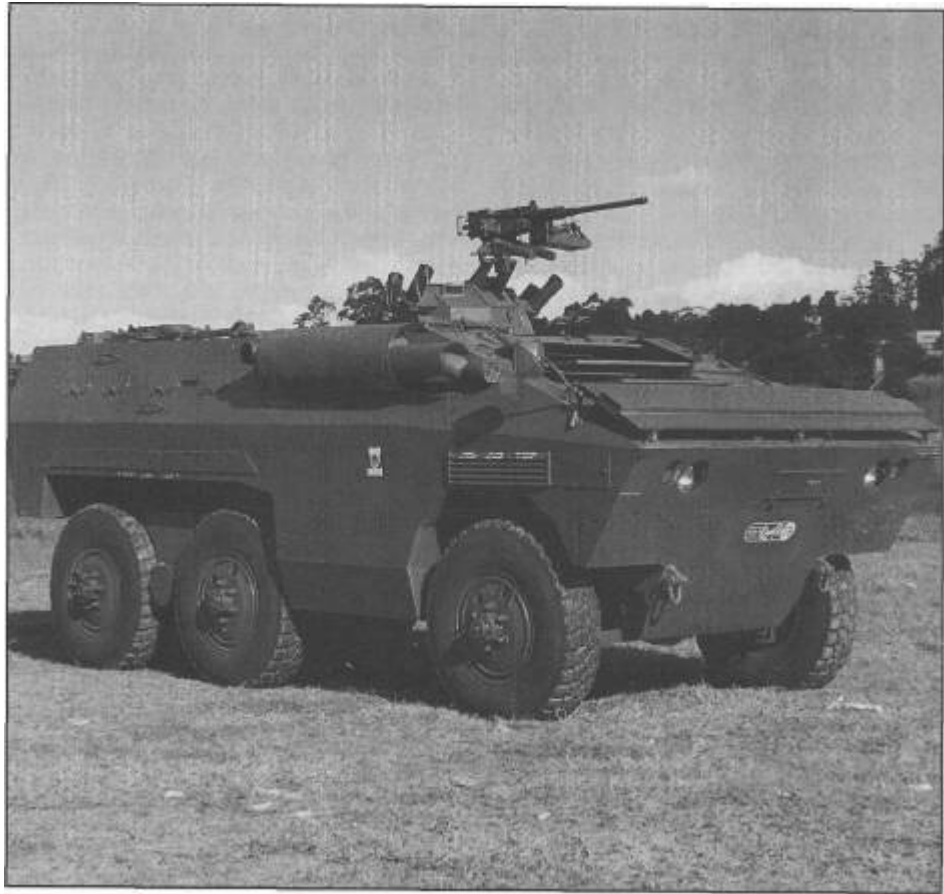
The Brazilian Urutu 6x6 APC seen here armed with a 12.7mm MG.
