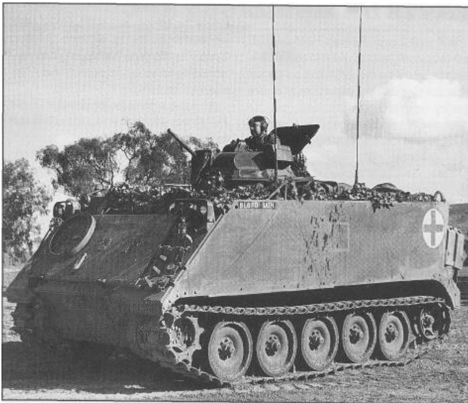
An Australian Army M113A3 APC, one of the many users of the most ubiquitous APC in the West.
