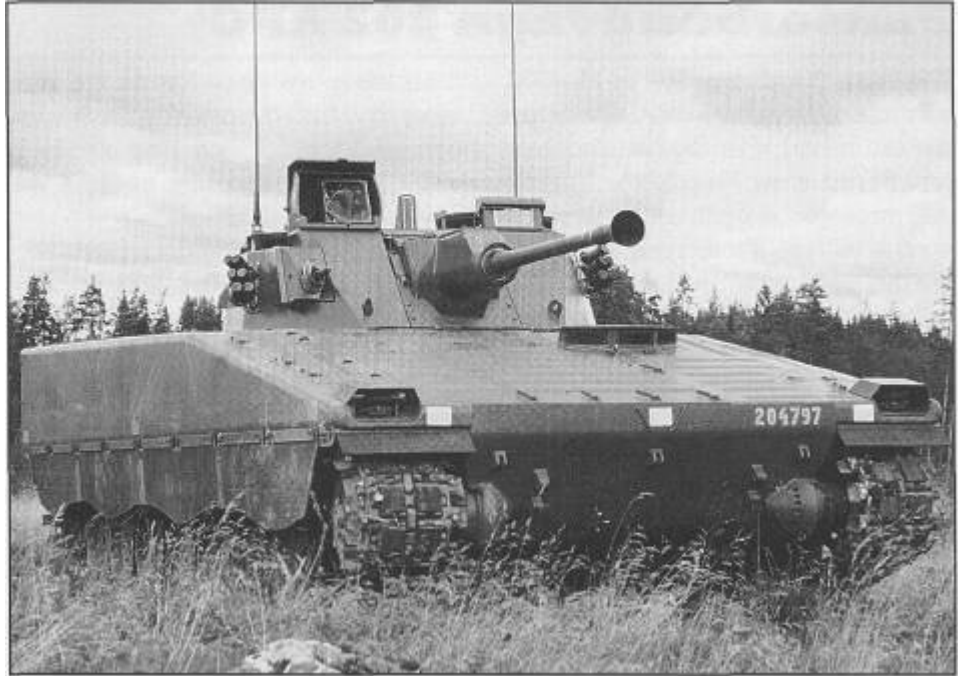
CV-90IFV armed with a Bofors 40 mm gun as the main armament.
