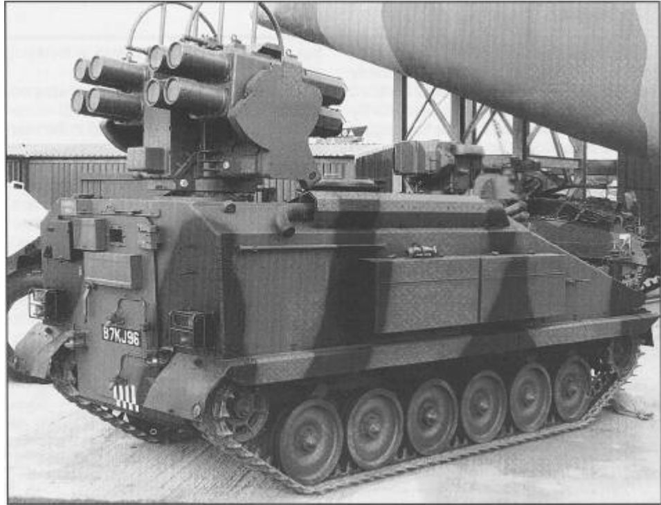
A Stormer APC configured as the carrier for the Starstreak air defence missile system.
