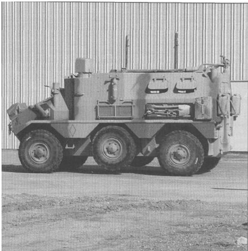
Side-on view of a Panhard VCR TTAPC-note the raised centre wheels.
