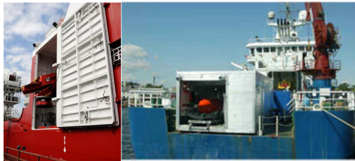
Figure 1 ROV LARS system (left, image courtesy of Cargotec) and UUV in containerised LARS (right, image courtesy of Kongsberg)
