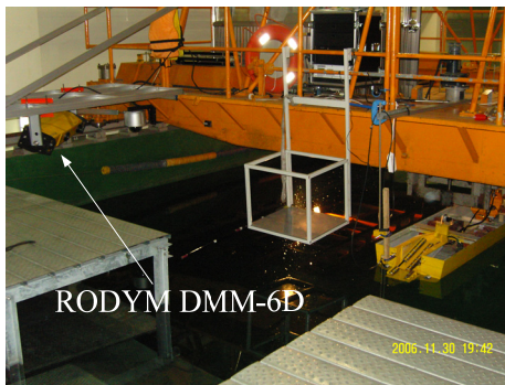
Fig. 7 6-D motion optical tracking system (RODYM DMM-6D) on the towing carriage.
