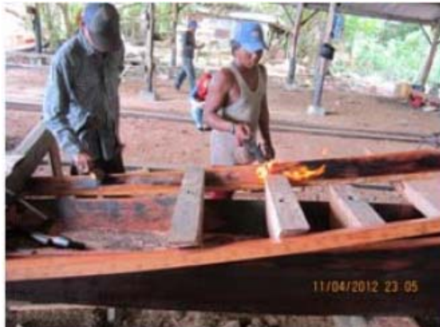
Figure 24: Hot bending technique
