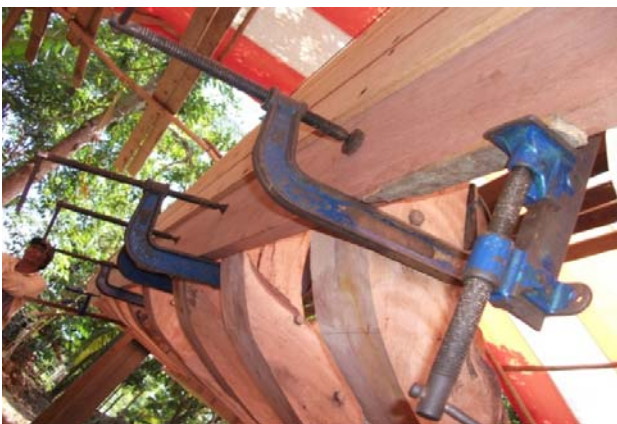
Figure 22: Clamp is used to hold the strakes
