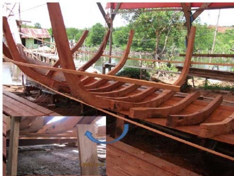
Figure 16: Longitudinal main stiffener
