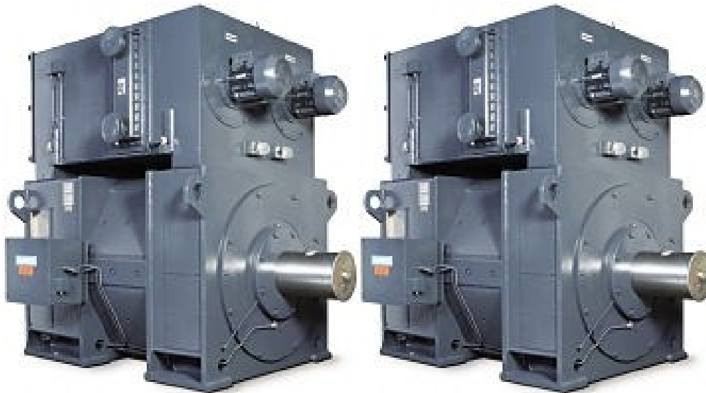
Figure E.1. TEWAC generator showing frame mounted fans and integral water to air heat exchanger.
