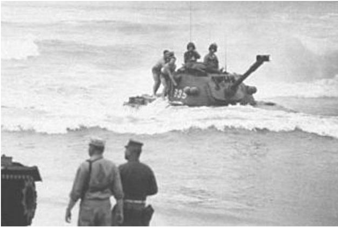
This M48A3 with a deep water fording exhaust stack attached on the rear coming off a landing craft on 7 September 1965. Note the support cable attached to the exhaust stack.
