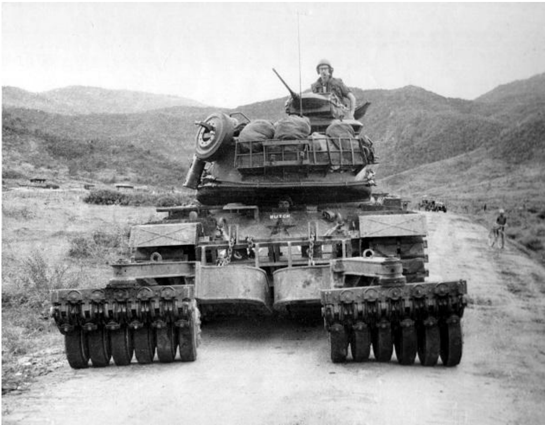
This M48A3 has added some additional protection. The large umbrella protected the turret crew from the pouring rain and the hot sun. For additional firepower, twin M2 Browning .50 Caliber MGs with flash suppressors was mounted on top of the commander's copula.
