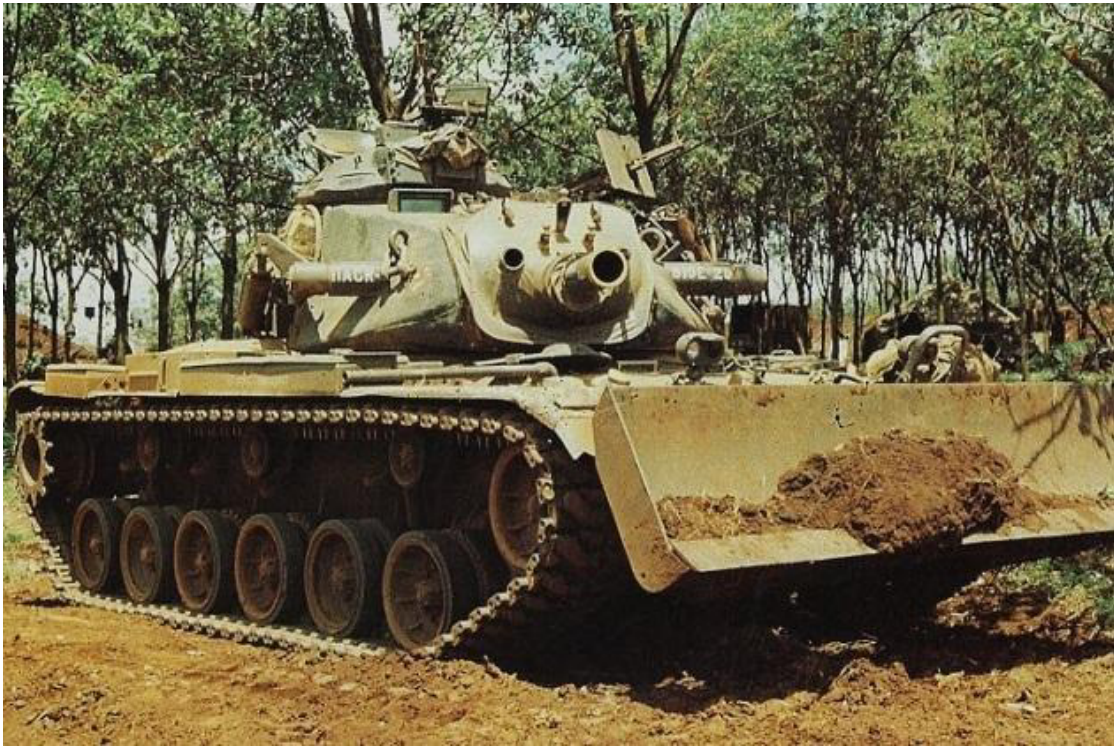
This M48A3 named "Wild One 4" was operated by the 919th Engineers as additional protection while brush clearing, building bridges and especially when clearing the roads of mines which were under the constant threat of an ambush.
