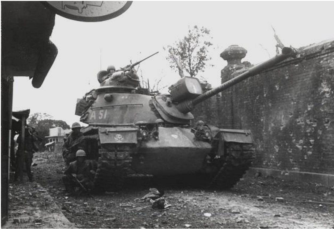
This is the left side view of the M48A3 number A51. Note the Citadel wall to the left and on the tank the double Jerry cans mounted on the turret and the ammunition can and two Jerry cans on the rear fender.
