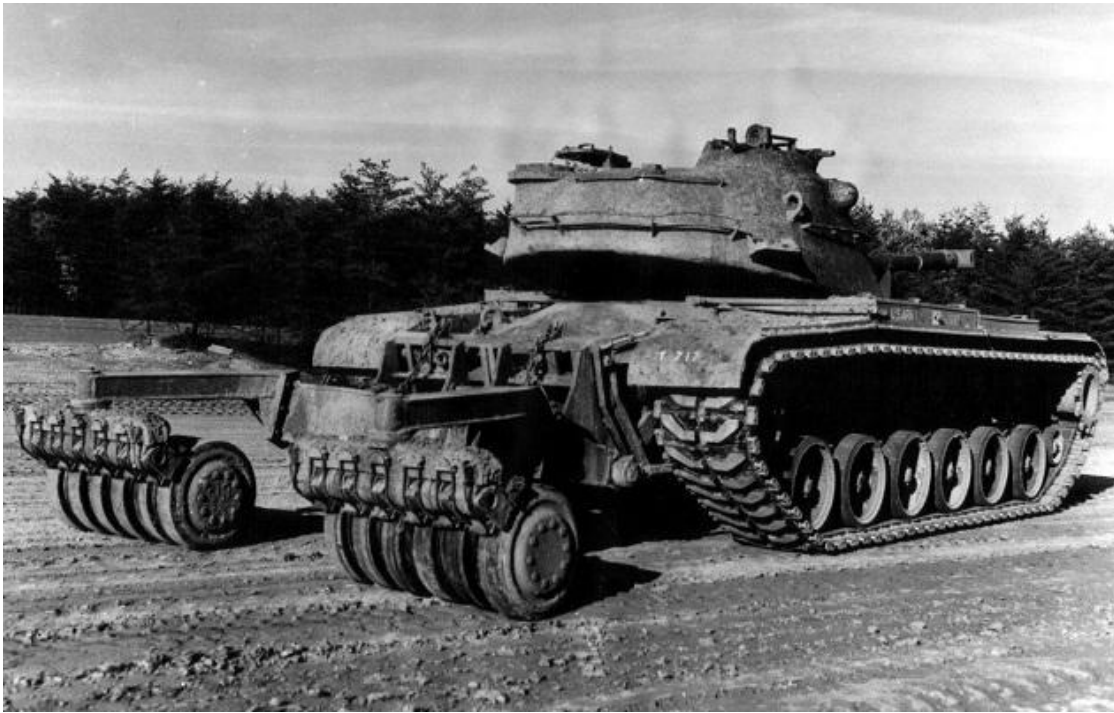
This M48A3 equipped the ENSURE 202 mine roller was operating on Route 19 in August 1970. The name "Butch" is painted in front of the driver's hatch and note the star on the front hull was over painted black.
