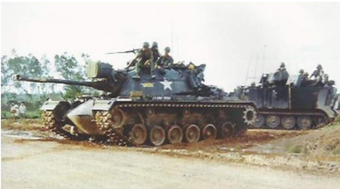
This another incorrectly captioned M48A2 attached to the 5th Infantry Division (Mechanized) moving up a beach in the Quang Tri Province during Operation Fisher on 6 January 1969. Note the unusual length of five track links on the side of the turret.
