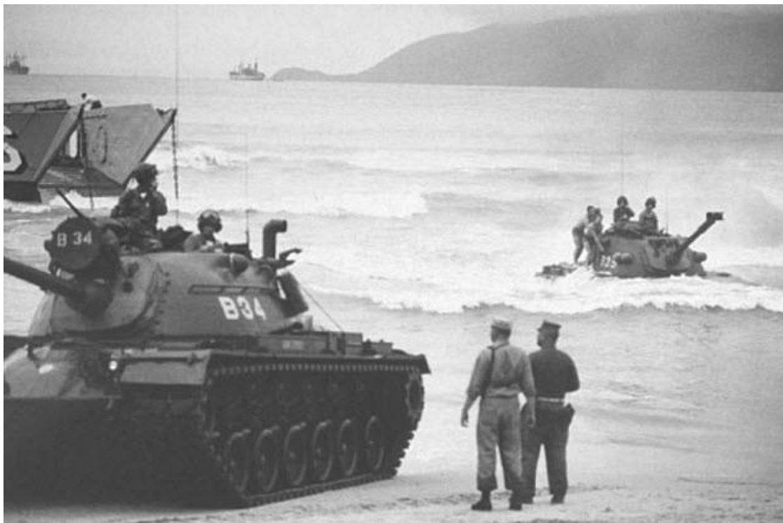
Tank B33 was launched into water above the fording depth of the tank and struggles to come ashore through the surf. Note that the water is covering the driver's hatch.
