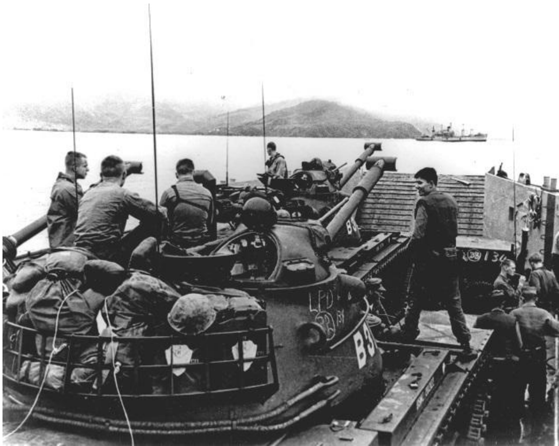
M48A3s equipped with deep fording kits wade ashore from the beached LCU.
