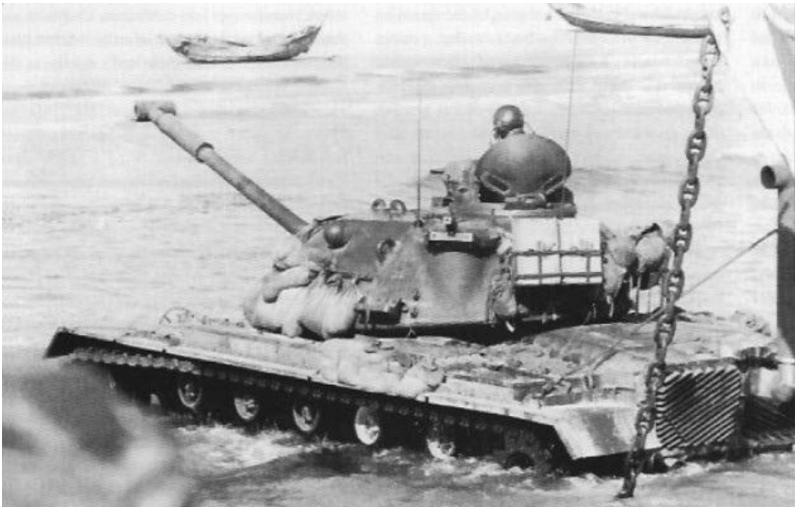
This M48A3 with a deep water fording exhaust stack attached on the rear coming off a landing craft on 7 September 1965. Note the support cable attached to the exhaust stack.
