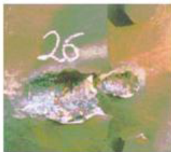
Fig. 6. Crater in plate of RHA armour after firing ERAWA-2 cassette from tank, with 125 mm projectile BM-15 (APFSDS-T, h = 300 mm, \alpha = 60^\circ ). Penetration of RHA armour h_w = 130 mm, protective ability of cassette CP = 57\%
