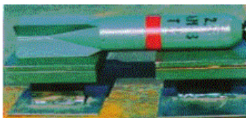
Fig. 17. Scheme of resistance test of ERAWA-1 cassette to detonation and destruction during burning of incendiary bomb ZAB-2,5 containing thermite (3000 °C) on it
