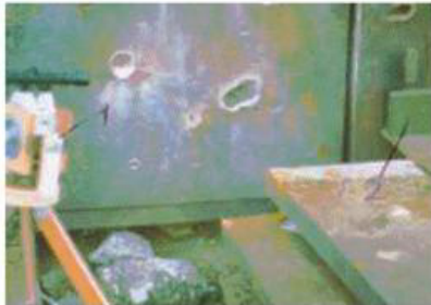
Fig. 7. Scheme of test of protective ability of ERAWA-2 cassette (2) by firing with the use of EFP warhead (1) ( d = 100 mm, h = 85 mm), ( \alpha = 60^\circ )
