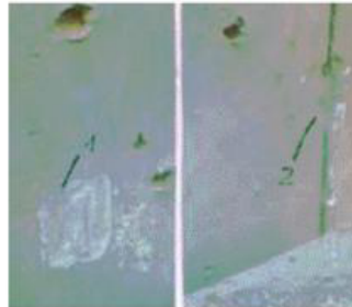
Fig. 8. Traces on RHA armour after penetration of ERAWA-2 cassette with warhead EFP; 1 - trace of detonation of ERAWA-2 cassette, 2 - trace of destroyed EFP projectile (EFP - h = 85 mm), h_w = 5 mm, protective ability of cassette CP = 94\% , ( \alpha = 60^\circ )
