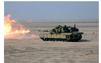
An M1A1 Abrams, firing its US built M256 120 mm tank gun
