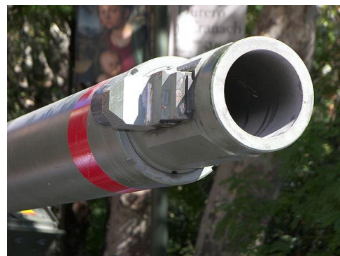
Muzzle of a Rheinmetall 120 mm L/55 tank gun on a Spanish Leopard 2E
