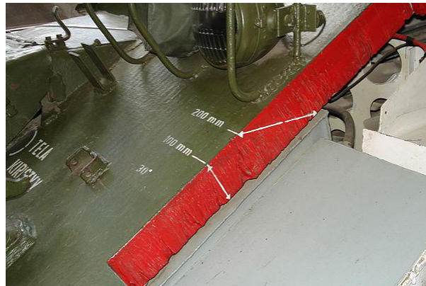
Sloped armour on the front of Soviet T-54 tank, here cut open to demonstrate the increase in effective thickness.
