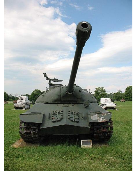
The extremely late-war-designed Soviet IS-3 utilized a pointed prow in place of a simple glacis
