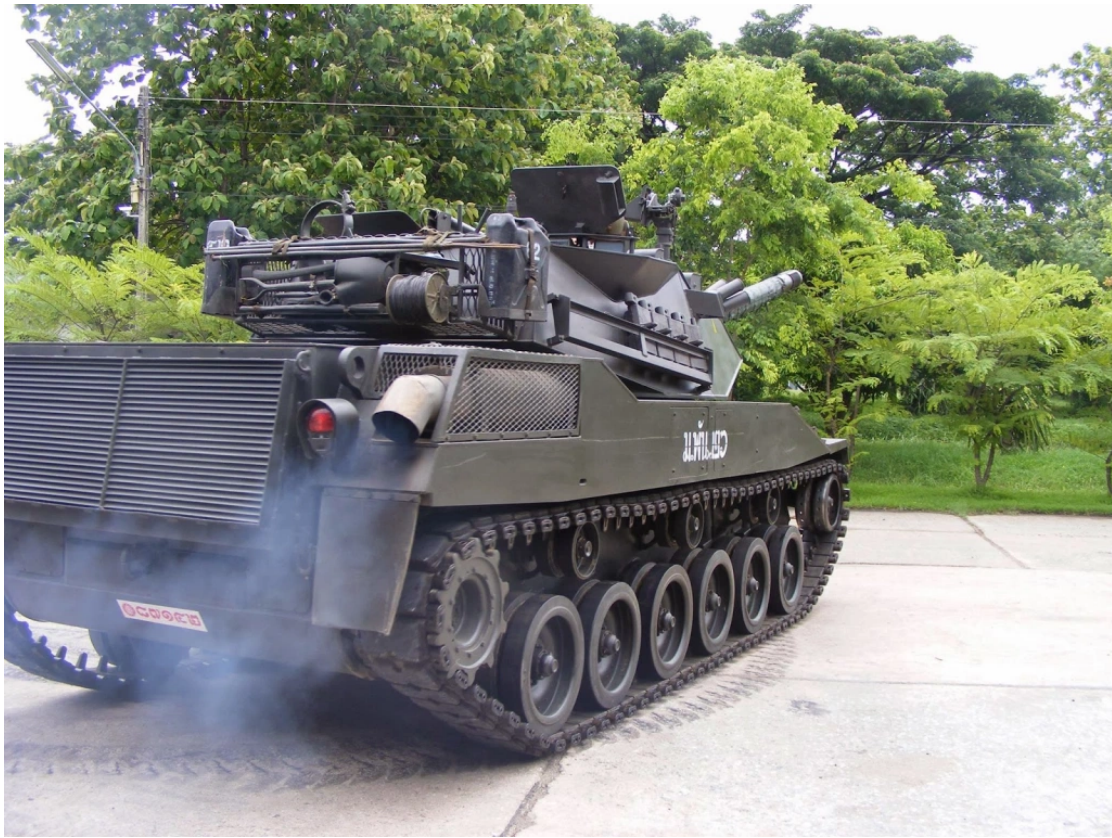
Exhaust outlet on the right side of the hull - Image @thaidefense-news.blogspot.com
