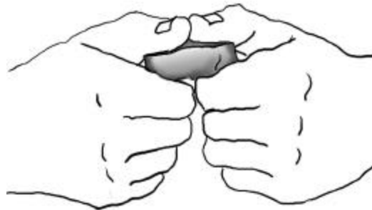
Figure A2.1. Proper Handling for Breaking or Dry Strength Test.
