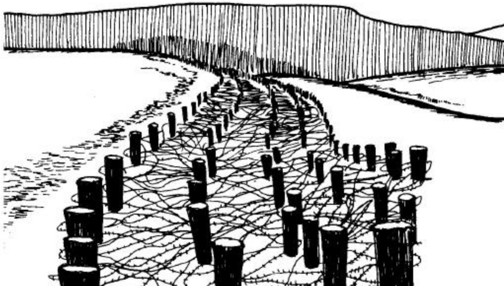
Figure 53. Posts and Entanglements along Roadway.
