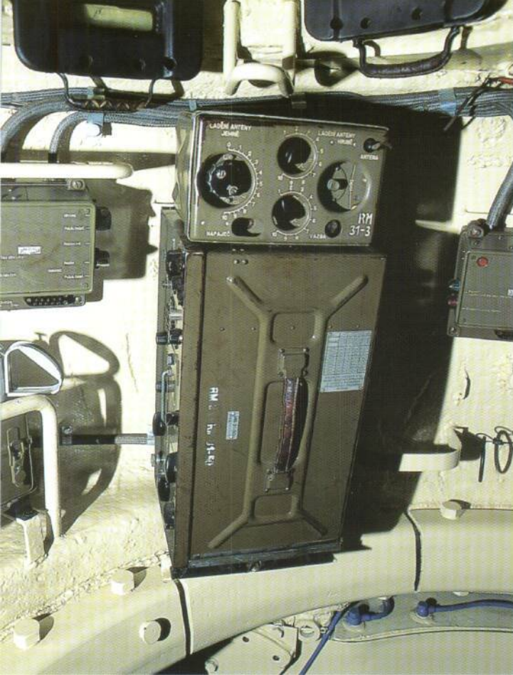
(Left) The radio equipment in this ex-Czech Army tank is of Czechoslovak manufacture, but installed in the original position high on the left turret wall, convenient to the commander's hand. Two of the cupola vision blocks are seen above it.
