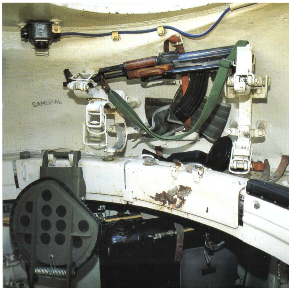
(Left) Looking from gunner's station to right rear of the turret, under the loader's hatch; the AK is jammed behind a clip for 100mm ammo. The turret looks deceptively roomy - it is in fact very cramped, especially when the (still inadequate) load of 43 x 100mm rounds are stowed.
