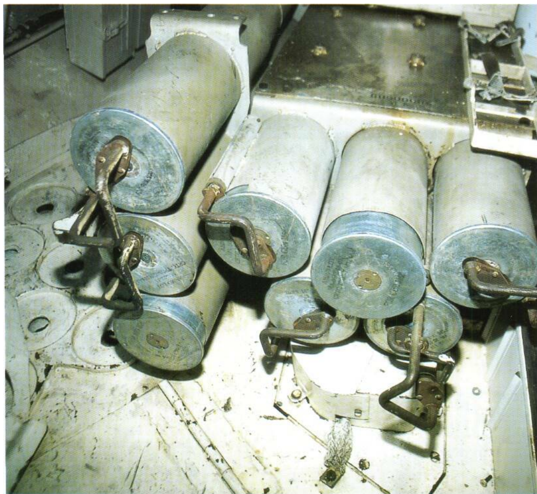
(Above & right) Radio installation and some of the ready ammunition stowage in an M60A1 turret bustle. These protective tubes for individual 105mm rounds are fitted wherever there is room for them, including 26 flanking the seat in the driver's compartment; in all 63 rounds are carried for the main gun, plus 900 for the .50cal machine gun in the TC's cupola, and another 5,950 for the 7.62mm coaxial gun. The turret is spacious and well laid out, with room for even tall crewmen to stand up comfortably; its format is conventional, with the loader on the left of the gun beneath his own roof hatch, and the gunner sitting ahead of the TC's knees on the right.
