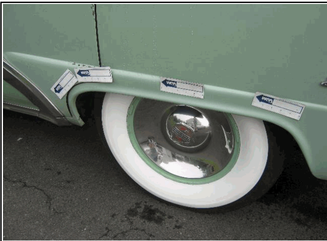
Picture Description : Quarter Panel Cracked Over 12"
