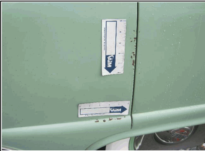
Picture Description : Quarter Panel Cracked Over 12"
