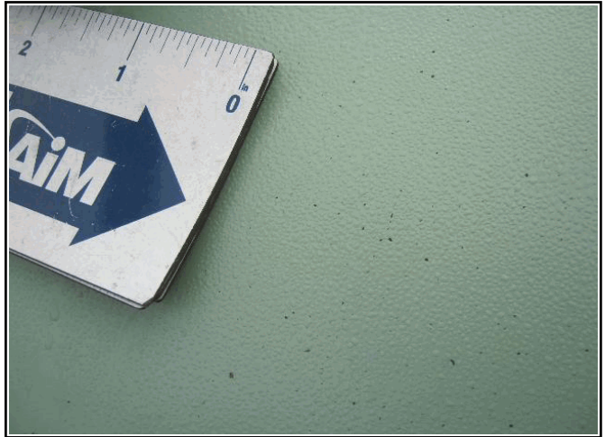
Picture Description : Fender Panel Chipped Minor
