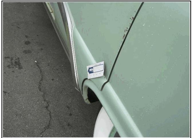
Picture Description : Quarter Panel Cracked Over 12"
