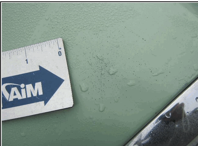
Picture Description : Fender Panel Chipped Minor
