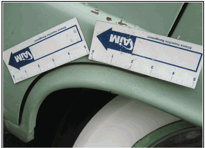
Picture Description : Quarter Panel Cracked Over 12"
