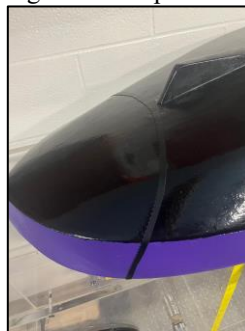
Figure 9. Hama strips on MTC bow
